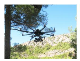
The *SmartAnalog* radio-controlled multicopter has eight propellers and a digital camera. The system can be operated by two people: a pilot and a camera operator equipped with a video viewfinder which displays the frame being shot in real time.
